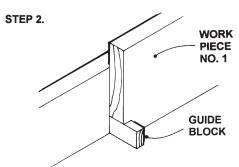
Step 2: Remove the spacer and move the workpiece over until it rests snugly against the spacer block.
