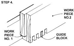
Step 4: Continue making cuts by placing the last notch cut over the guide block to position the boards for the next cut. Note: To ensure boards staying aligned together throughout the cutting process, use small c-clamps, if necessary.
