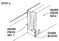
**Step 3:** Butt the 2<sup>nd</sup> workpiece tightly against the guide block, as shown. Then make a cutting pass to form the notch in both pieces simultaneously.
