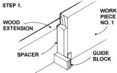
Step 1: Cut a spacer strip with dimensions that equal the groove width and insert it between guide block and 1st workpiece. Then, while holding the workpiece firmly, make the first cut.
