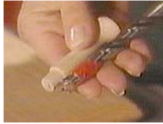
Mark the depth on the drill with some tape
