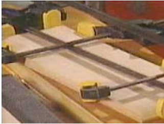
Clamp the pieces in place to dry
