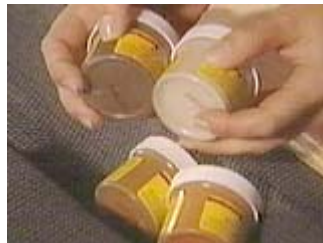
Oil-based filler comes in many colors and can be mixed together to achieve the correct shade
